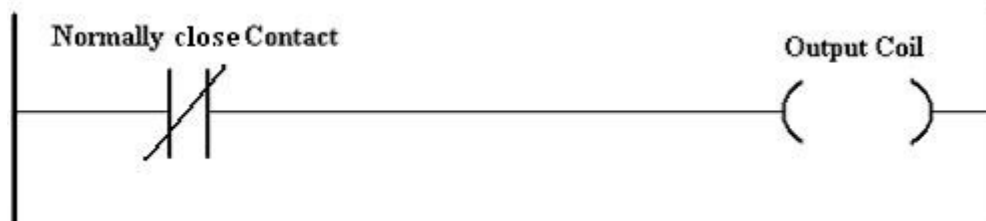
Figure 11. A rung contains a NC contact and an output.
