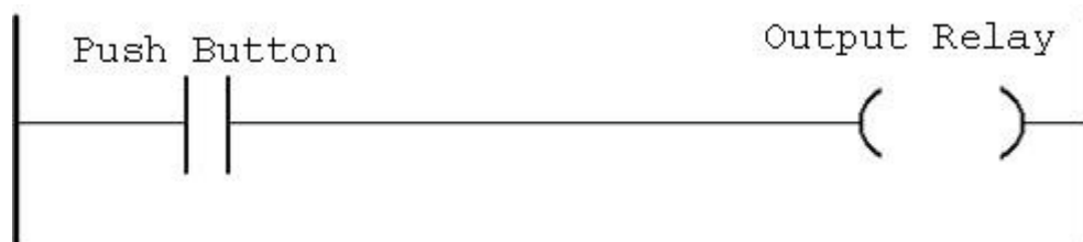
Figure 18. Pushbutton operates motor.
